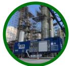
**Mobile incinerator with a combustion capacity of 4 MW**Our 4 MW unit is also perfectly suited for short-term deployments, especially for the degassing of single tanks and short back-up operations for stationary vapor recovery units (VRU).
