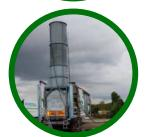
Mobile incinerator with a combustion capacity of 20 MW
